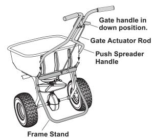
5. Secure the handle assembly with the 1/4" x 1-3/8" cap screws and 1/4" locknuts from the hardware kit.
