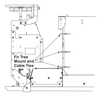
3. The strobe light kit contains two harness assemblies: 56" and 72". Determine your harness routing and connect the appropriate harness to each strobe light.
