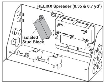
4. Connect the single-pin terminal on the relay/fuse assembly harness (yellow wire) to the white wire coming from port A of the spreader module.
