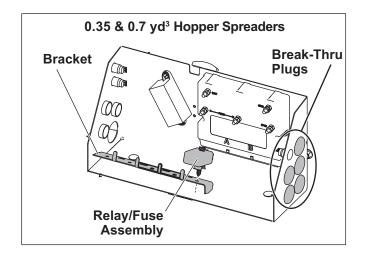
5. Remove a push plug from a mount hole on the electrical box and mount the relay/fuse by pushing the connector clip on the back of the assembly into the mount hole.
