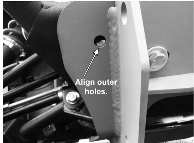
Verify that the skid plate assembly is centered left to right on the vehicle. Tighten the fasteners installed in Step 4.
