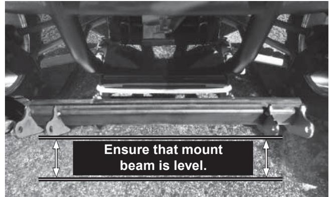
13. Choose the set of holes in the skid pan assembly that positions the mount as close as possible to 10-5/8" from the ground when measured as shown. Tighten the fasteners according to torque chart.
