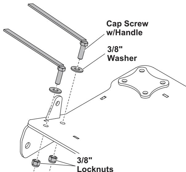
8. Reinstall the skid plate assembly using M10 x 1.25 x 30 fasteners. Make sure that the cap screws from Step 7 protrude through the corresponding holes in the skid plate assembly. Secure with locknuts, fastening them hand tight.
