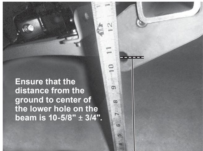
14. Measure the distance between the mount beam rear hole and the ground. If it exceeds 11-1/2", install the accessory Height Adapter Plate Kit (PN 77555) to ensure optimum plowing performance.
