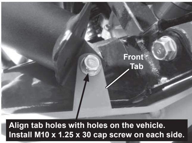
5. Clamp the rear of skid plate assembly to the vehicle frame.
