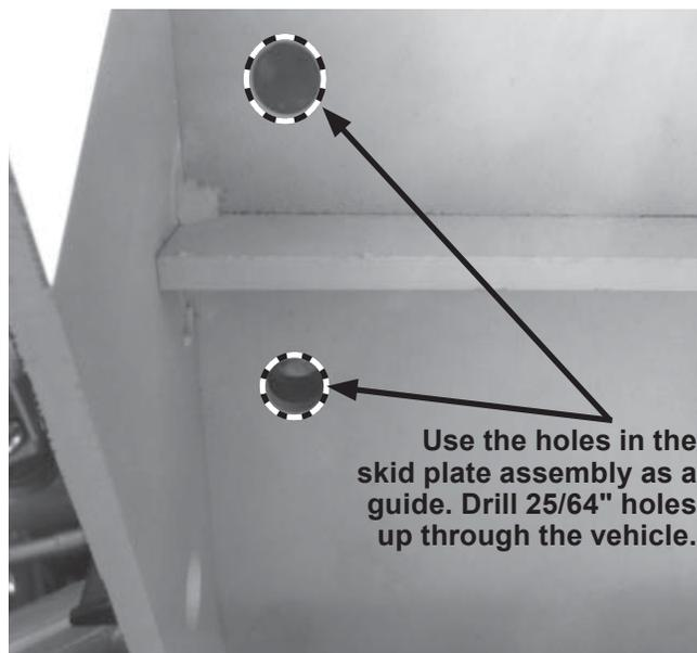
7. Remove the skid plate assembly. Place a washer on each of the four cap screws with handles. Insert them down through the holes drilled in Step 6.
