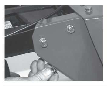
4. Use a 13 mm wrench to tighten the fasteners that hold the brushing mechanism to the axle drive housing. Tighten in the order shown.
