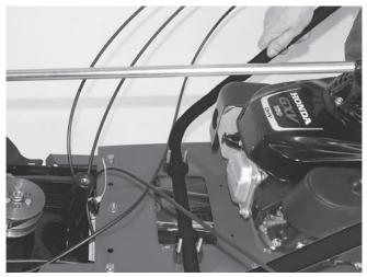
2. Mount handlebar to the supports with the knob.
