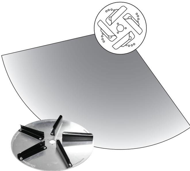
When looking down at the spinner, moving the fins counter-clockwise will adjust the spread pattern toward the right side of the spreader.
