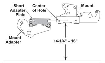
4. If the measured height is 16"–17-1/4", install the tall height adjustment adapter plates as described.
