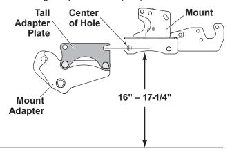
5. Position the adapter plate against the driver's side portion of the mount adapter as shown. Insert a 3/4" x 2-3/4" cap screw through the lower front adapter plate hole and through the appropriate hole on the mount adapter. Secure with a locknut.
