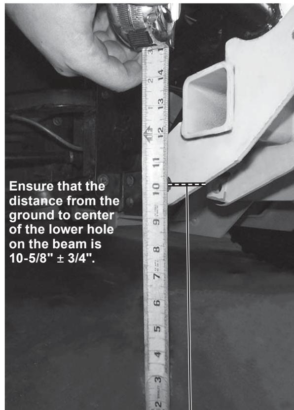
8. Measure the distance between the mount beam rear hole and the ground. If it exceeds 11-1/2", install the accessory Height Adapter Plate Kit (PN 77555) to ensure optimum plowing performance.
