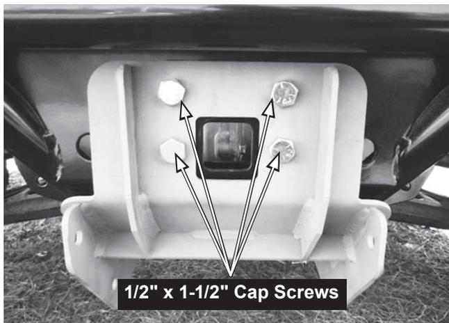
5. Place a 1/2" washer over each M12 x 50 cap screw. Insert the cap screws with washers up through the rear holes of the skid plate assembly and thread into the matching holes on the vehicle. Fasten hand tight.
