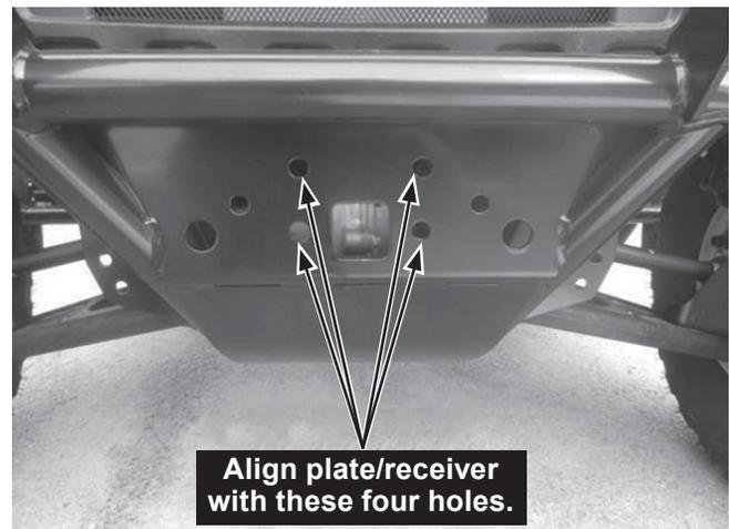
4. Insert a 1/2" x 1-1/2" cap screw into each of the holes. Secure with 1/2" washers and 1/2" locknuts. Hand tighten the locknuts.
