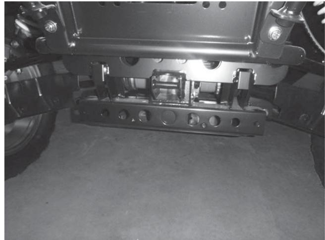
**For all Exmark, Toro, and 2014–15 Arctic Cat Models:** Remove the lower metal brush guard bolts; retain the fasteners for reinstallation.
