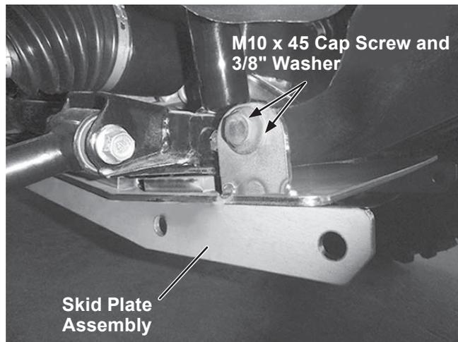
3. Align the four slots (two of which are shown in the photo below) in the bottom of the skid plate assembly with the weld nuts in the UTV frame. Insert an M10 x 45 cap screw and 3/8" washer into each skid plate slot and engage the weld nuts.
