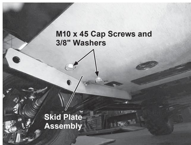
4. Tighten the cap screws (total of six) installed in Steps 2 and 3 to the recommended torque according to the torque chart.
