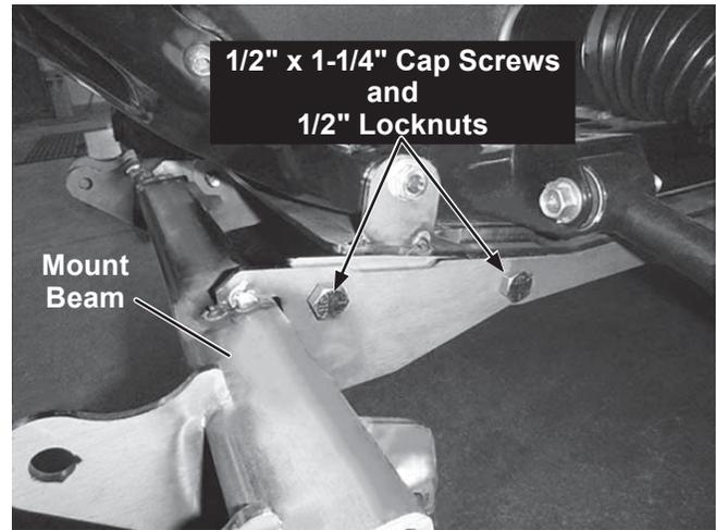
9. Measure the distance between the mount beam rear hole and the ground. If it exceeds 11-1/2", install the accessory Height Adapter Plate Kit (PN 77555) to ensure optimum plowing performance.
