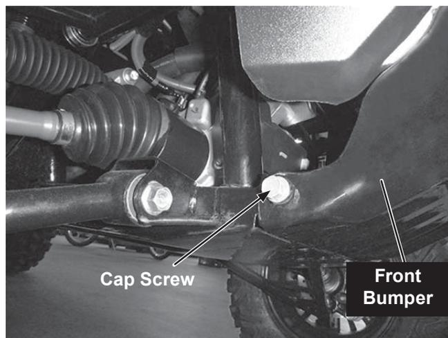
2. Position the skid plate assembly as shown below and secure it in place using an M10 x 45 cap screw and 3/8" washer on each side of the UTV. Do not fully tighten the cap screws at this time.
