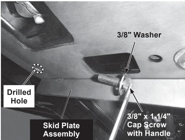
7. Secure the 3/8" x 1-1/4" cap screws with handle using the provided 3/8" locknuts.
