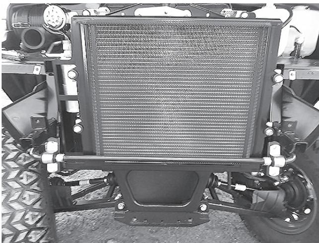
2. Remove the two carriage bolts that secure the top of the radiator frame. Remove the two carriage bolts that secure the bottom of the radiator frame.
