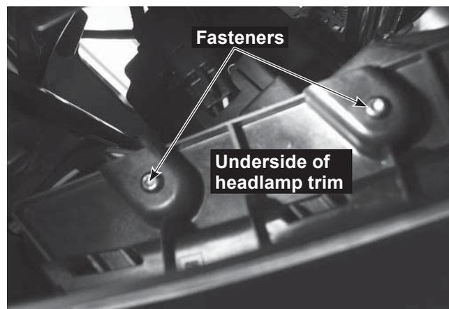
4. The headlamp is held in place by four fasteners. Remove the two fasteners on the top of the headlamp, as well as the fasteners on the side and the front.
