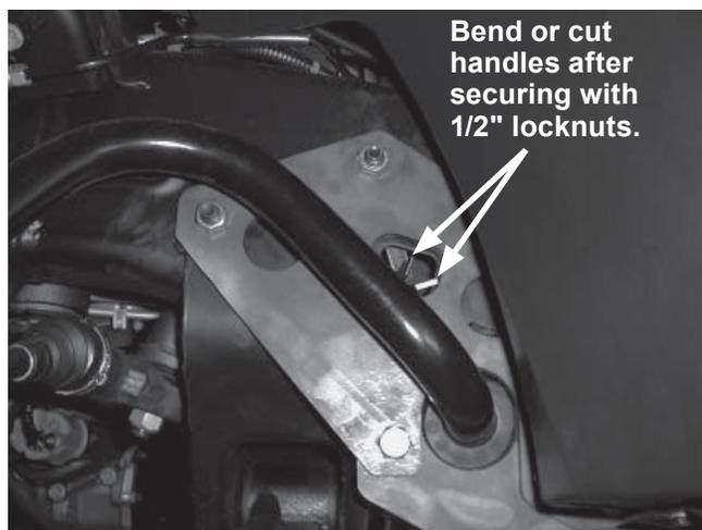
Repeat this process on the driver's side, noting that the rearmost cap screw with handle must be inserted through the round hole behind the rear bracket as shown. Bend or cut handles so that they do not interfere with the range of motion of the front stabilizer bar.
