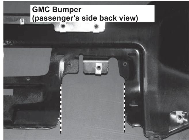
3. Remove the plastic portion of the bumper and notch as shown below.
