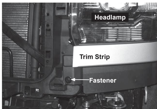
3. Remove the two fasteners on the underside of the headlamp trim.
