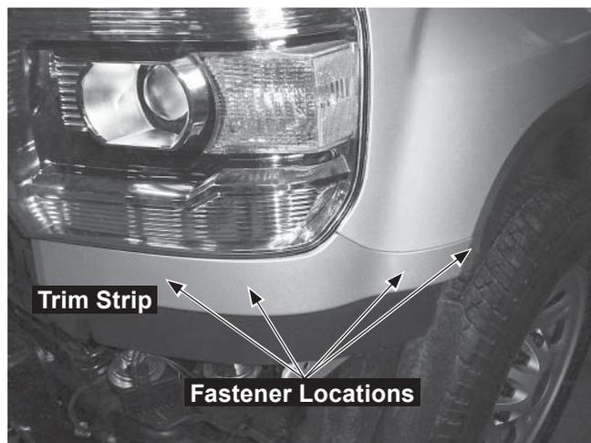
2. Remove the fastener to the side of the plastic trim piece. Remove the trim piece.
