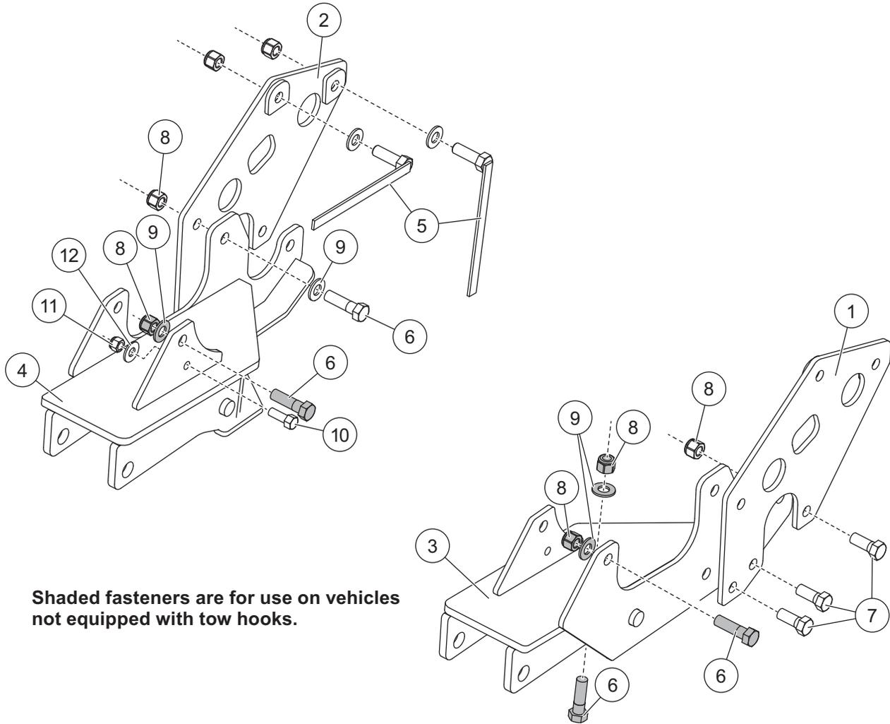
**Shaded fasteners are for use on vehicles not equipped with tow hooks.**
