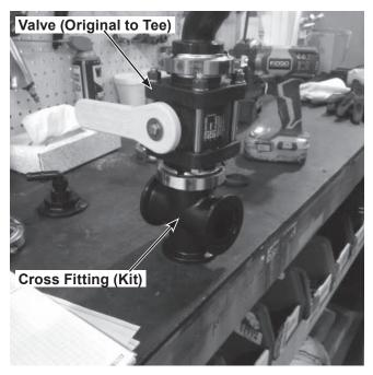
8. Install the 90° hose barb and adapter fitting from the reconfiguration kit into the opposite end of the cross fitting.
