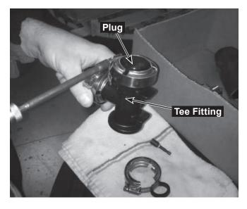
4. Install the plug on the large tee fitting remaining at the top of the unit.
