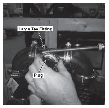
5. Remove the tee fitting located directly above the pump. This may require loosening additional clamps.
