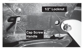
13. Bend or cut the ends of any cap screw handles protruding out from the truck frame, for appearance and to prevent contact with the sway bar.
