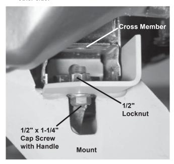
NOTE: For a more professional appearance, install the cap screws with the handles pointing in toward the center of the vehicle.
