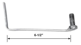
12. On both sides of the vehicle, insert a 1/2" x 1-1/4" cap screw with bent handle into the side of the frame, and pass it out through the drilled 17/32" hole and the hole in the rear of the mount. Place a 1/2" locknut on each of the cap screws, and fully tighten according to the torque chart.
