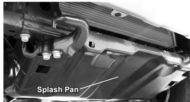
4. Slide the mount into place with the rear arms behind the front cross member and above the splash pan. Align the bottom slots in the front of the mount with the end cap holes in the bottom of the front cross member, and clamp the mount in place.
