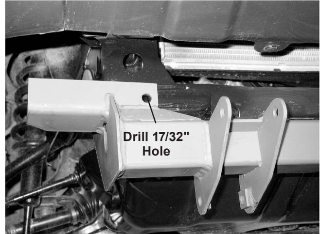
7. On both sides of the vehicle, place a washer onto one of the bolts with the shorter handles, and pass it into the end of the front cross member and out through the drilled 17/32" hole and the hole in the front of the mount. Place a locknut onto each of these bolts, and fully tighten according to the torque chart.
