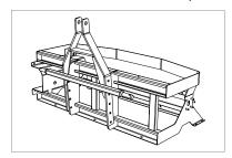
2. Align the bolt holes; fit the bolts through from the outside.
