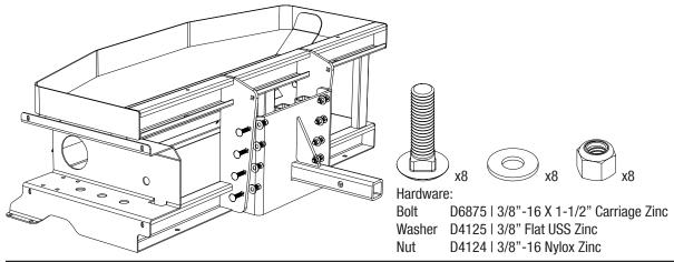
**STEP 2** Insert the hitch into the vehicle's receiver. Lock with the Hitch Pin (D4136) and Hair Pin.
