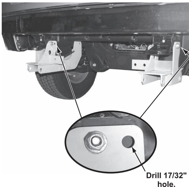
6. Using the rear holes in the passenger-side mount as a guide, drill two 17/32" holes into the truck frame.
