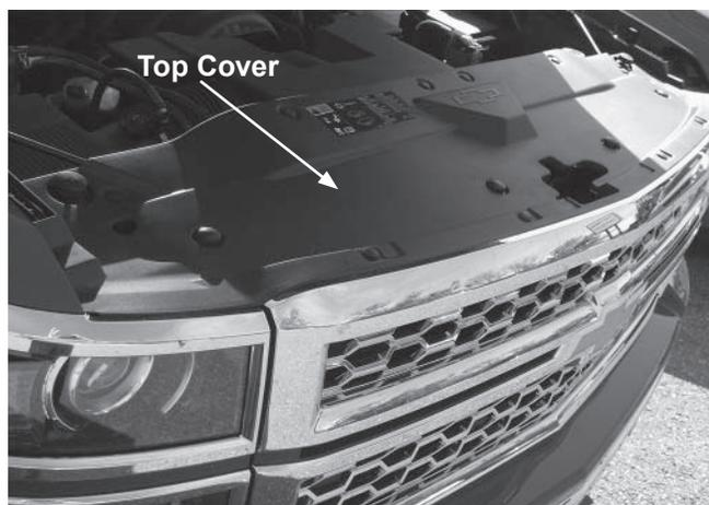
2. Remove the four cap screws and release the locking tabs located along the top of the grille.
