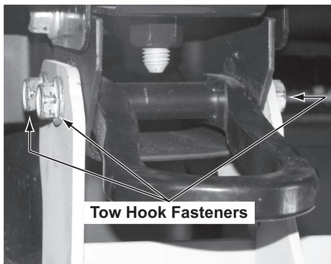
3. Attach the passenger-side mount and tow hook to the truck frame using the original tow hook fasteners. Hand tighten.
