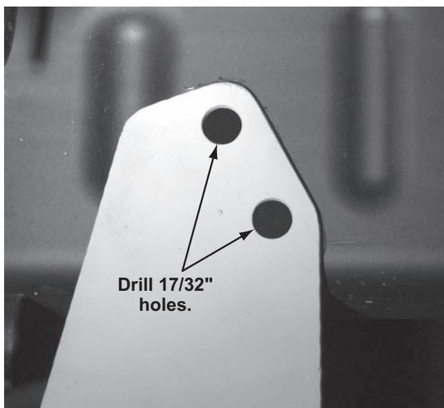
7. Insert two 1/2" x 1-1/4" cap screws with handles and 1/2" flat washers into the inside of the truck frame and out through the rear drilled holes. Attach a 1/2" locknut to each cap screw and hand tighten.
