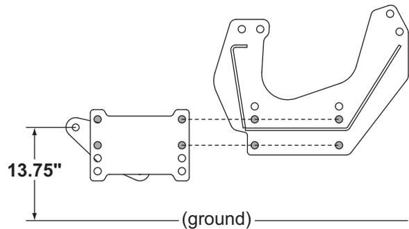
14. Attach the pushbeam to the mount plates using eight 1/2" x 1-1/4" cap screws. Place a 1/2" locknut on each cap screw, and fully tighten according to the torque chart.
