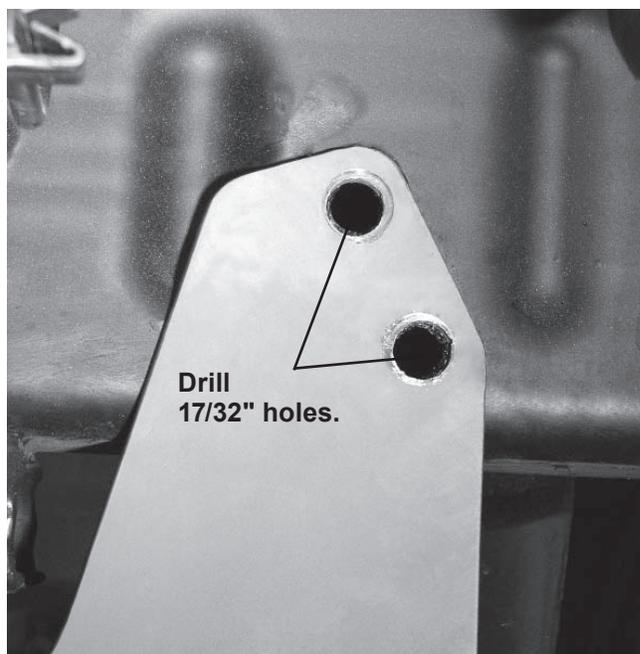
4. Insert two 1/2" x 1-1/4" cap screws with handles and 1/2" flat washers into the inside of the truck frame and out through the rear drilled holes. Attach a 1/2" locknut to each cap screw, and hand tighten.
