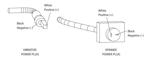
\* NOTE: Plug has polarity reversed for proper motor rotation
