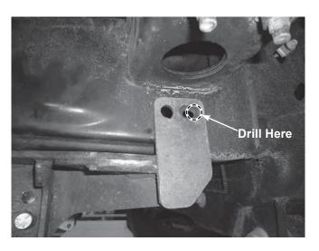
7. Attach a 1/2" washer to each of two 1/2" x 1-1/2" cap screws with handle and insert them into the frame rail through the opening shown and then through the mount holes. Start with the front mount hole to ensure that the rear fastener handle will not block access.
