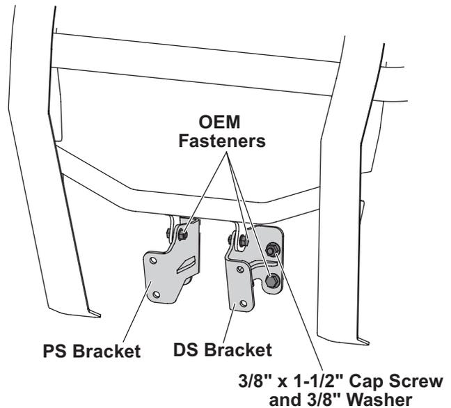
**NOTE: The bracket flanges should point outward and the center fastener hole should be on top.**
