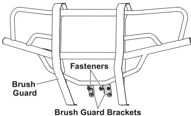
2. Use the OEM fasteners and two each of the supplied 3/8" x 1-1/2" cap screws, 3/8" washers, and 3/8" locknuts to install the supplied driver-side and passenger-side brackets and frame brackets in place of the lower brush guard brackets. Skip ahead to Step 5.
