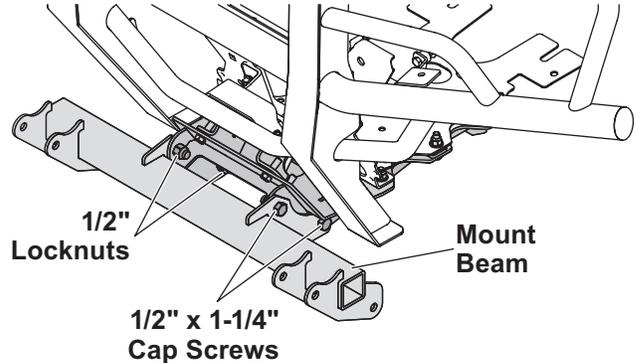
**NOTE: The plastic guard may require trimming to avoid interference with the mount beam as shown.**
