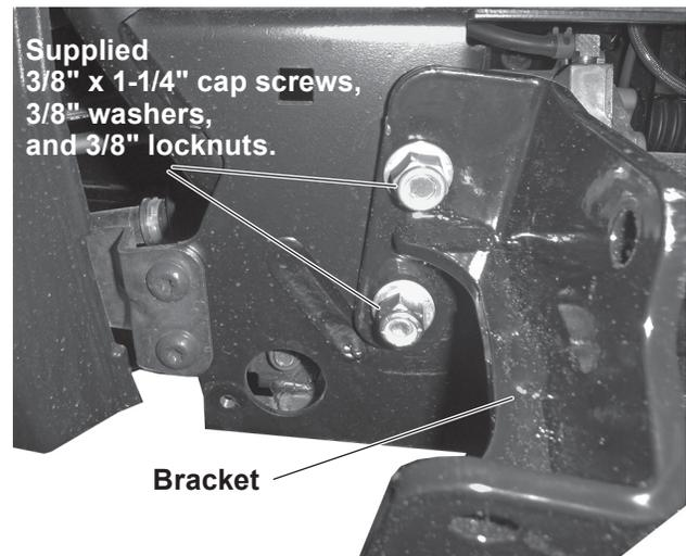
5. For all applications, position the skid plate assembly on the brackets as shown. Secure the skid plate assembly to the brackets with four 3/8" x 1-1/4" cap screws and four 3/8" locknuts.
