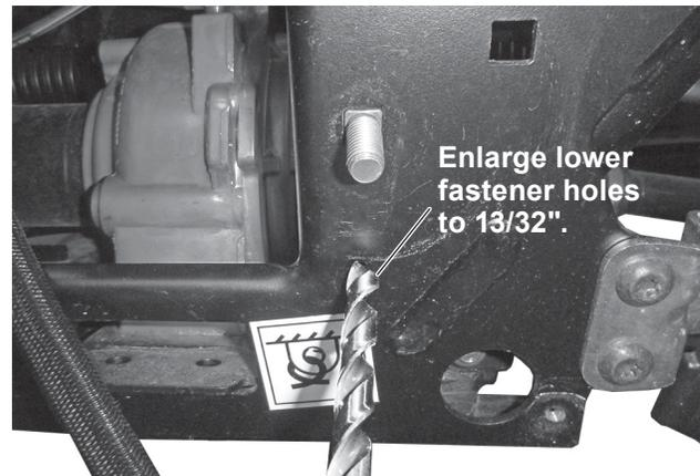
4. Using four of the supplied 3/8" x 1-1/4" cap screws and 3/8" washers, install the supplied driver-side and passenger-side brackets to the front of the frame. Secure each cap screw with a 3/8" washer and a 3/8" locknut.
