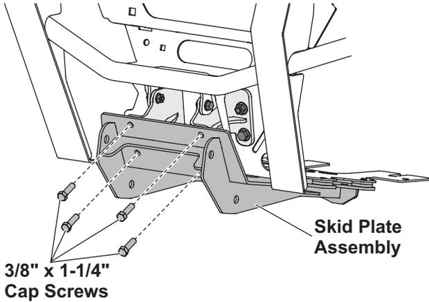
6. Install a 3/8" x 1-1/4" cap screw with a 3/8" washer through the two front skid plate attachment holes. Secure with 3/8" washers and 3/8" locknuts.
