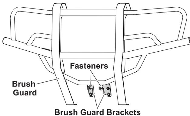
2. Use the OEM fasteners to install the supplied driver-side and passenger-side brackets in place of the lower brush guard brackets. Skip ahead to Step 5.
