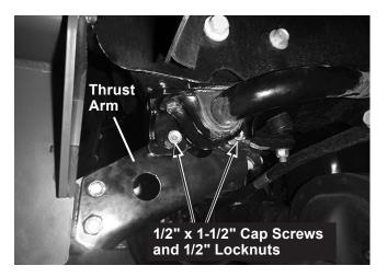
Remove the driver-side and passenger-side stabilizer bar bracket bolts. Save stabilizer bar bracket bolts for reinstallation if the mount is removed.
