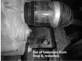
7. Place a 3/8" washer on each of two 3/8" x 3" cap screws. Install the cap screws with washers down through the driver-side brush guard bracket as shown.
