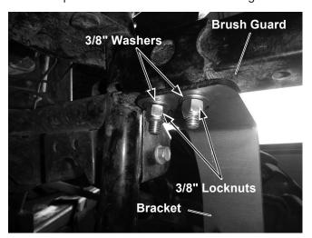
9. Place a 3/8" washer on each of two 3/8" x 1-1/4" cap screws.
