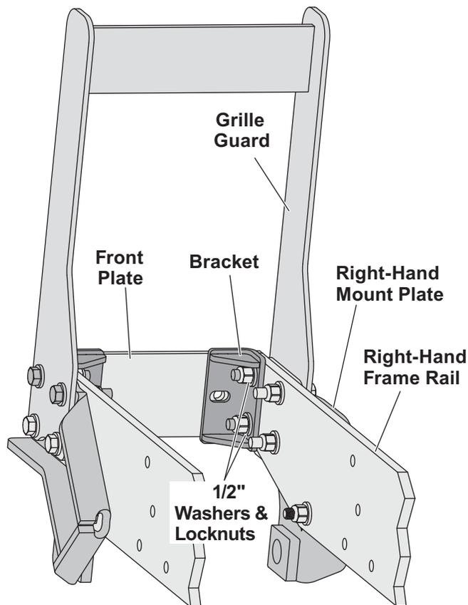
8. Place the front mount plate against the front frame plate of the tractor. Install two 1/2" x 2" cap screws through the holes of the mount plate and out through the brackets. Secure the cap screws to the brackets with 1/2" washers and 1/2" locknuts. Hand tighten.
