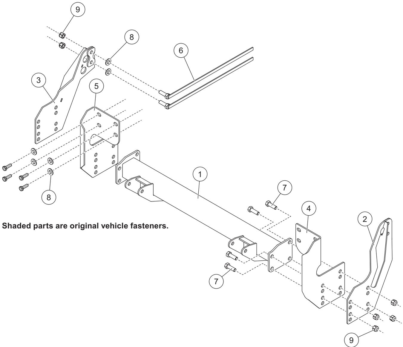
Shaded parts are original vehicle fasteners.
