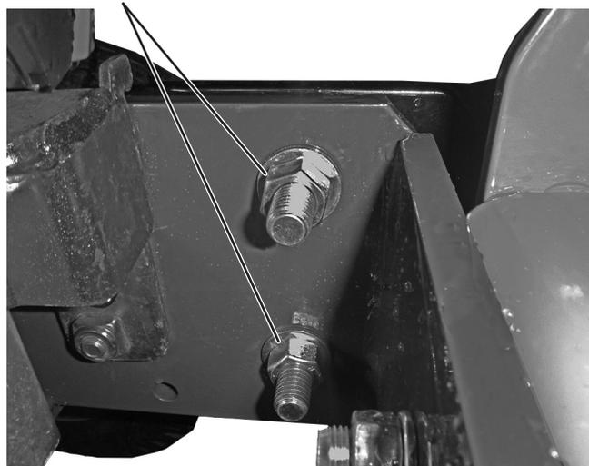
3. Install one 3/8" x 2-1/2" cap screw through the middle hole of the left hand side plate and frame rail as shown. Secure with a 3/8" washer and 3/8" locknut and hand tighten.
