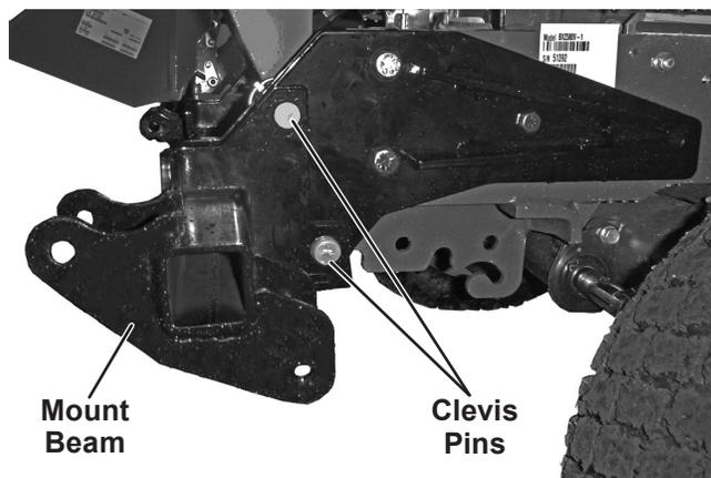
**NOTE: After five to ten hours of snowplow usage, retorque all mount assembly fasteners.**
