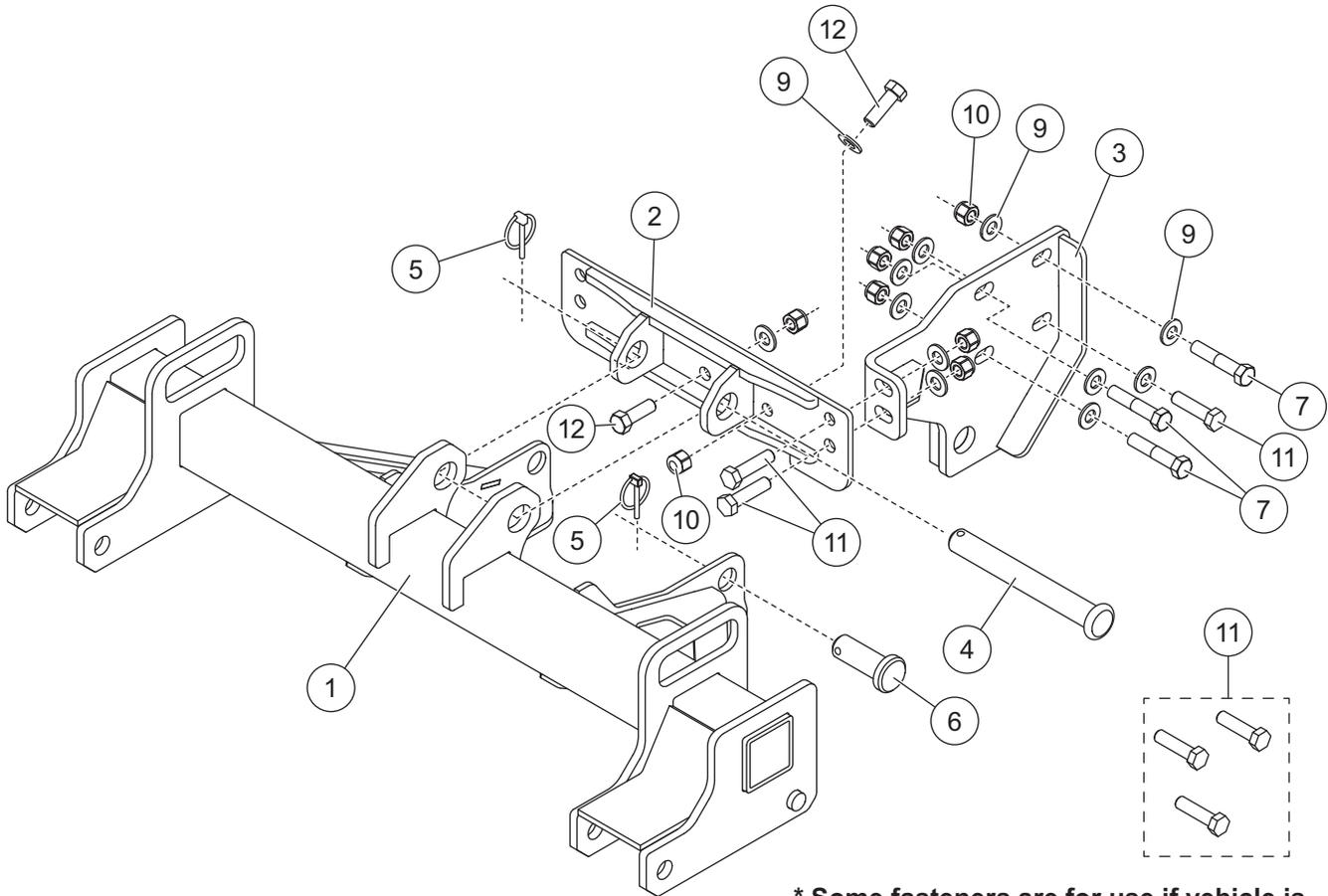
\* Some fasteners are for use if vehicle is not equipped with a brush guard. Refer to Installation Instructions for details.
