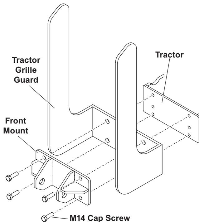
5. Tighten the fasteners according to the torque chart. Skip ahead to Step 9.
