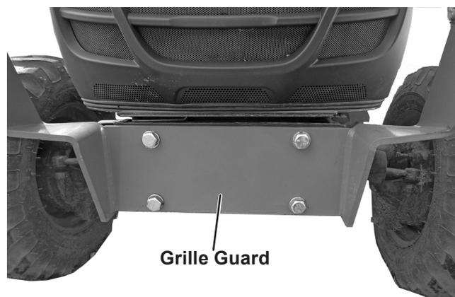
4. Place the front mount against the grille guard with the mounting holes aligned. Install the four provided M14 fasteners through the front mount, grille guard, and into the grille guard mounting holes.
