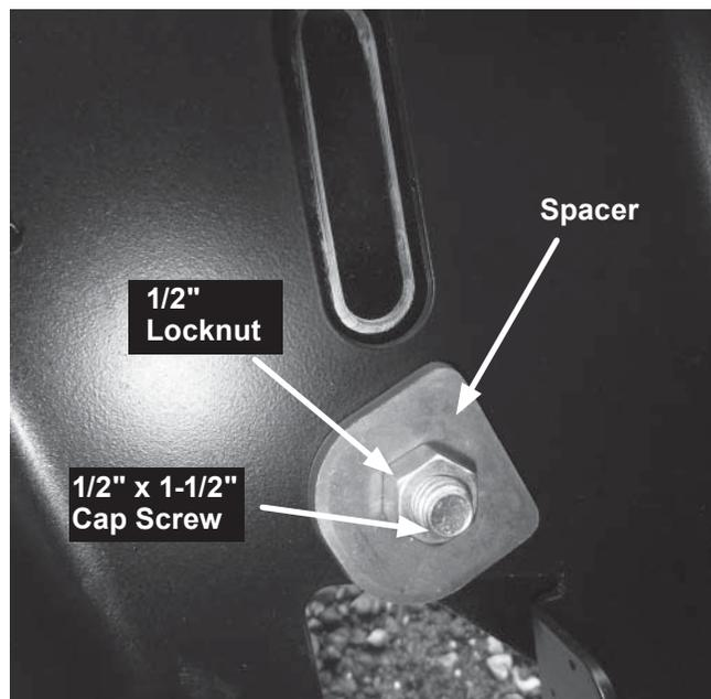
5. Tighten the fasteners installed in Steps 3 and 4 according to the torque chart.
