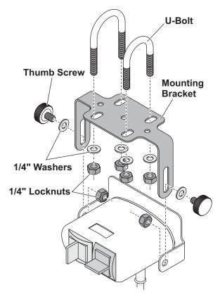
2. Attach the control to the slots in the bracket with two 1/4" thumb screws, two 1/4" washers, and two 1/4" locknuts as shown.
