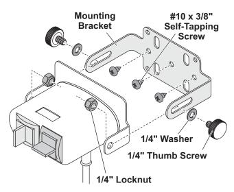
2. Attach the control to the slots in the bracket with two 1/4" thumb screws, two 1/4" washers, and two 1/4" locknuts as shown.
