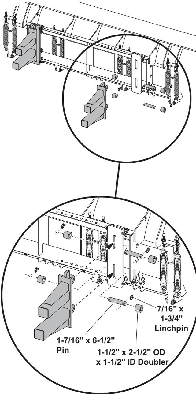
**NOTE:** Hardware and coupler mounting hubs shown in the image above are not included in the attachment plate kit. They are shipped with the pusher plow.
