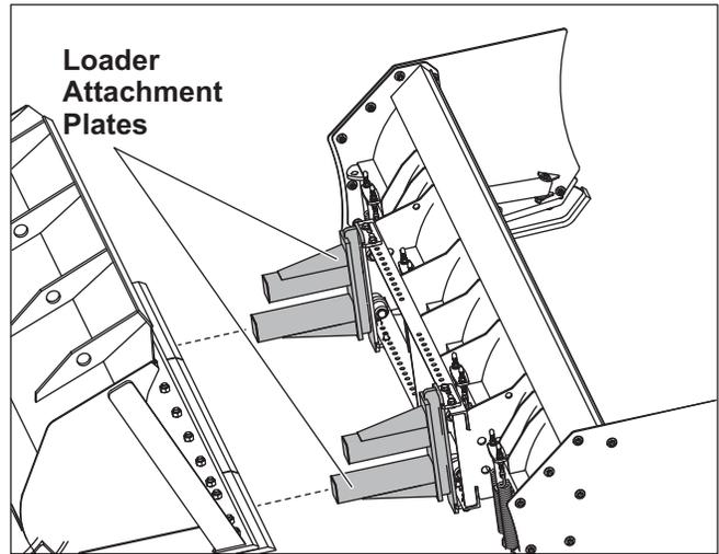
The bucket edge will rest against the attachment plates. The upper posts will fit inside the bucket and should be centered. The lower posts will be positioned under the bucket.
