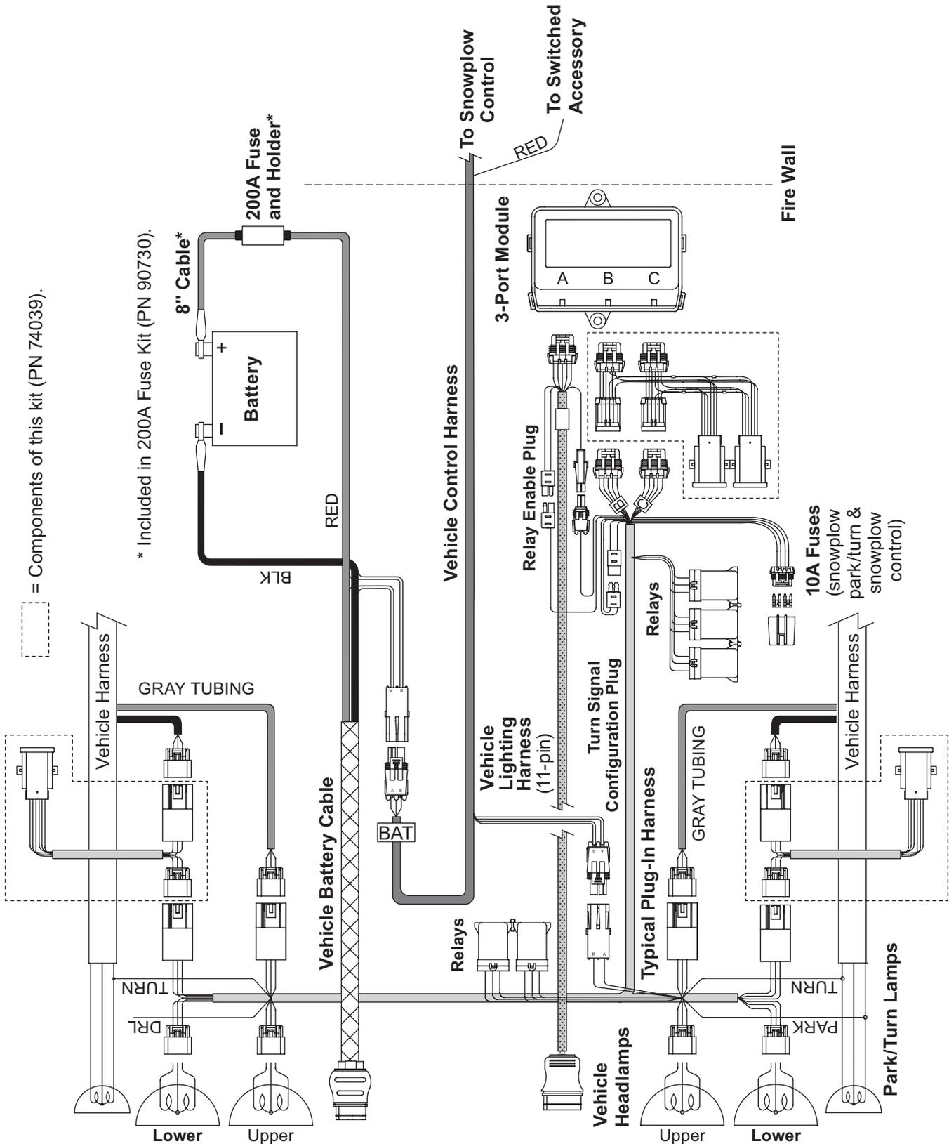
**TYPICAL LED PLOW LIGHT, HEADLAMP CONTROL MODULE (HCM), AND HARNESS DIAGRAM WITH 74039 ADAPTER KIT INSTALLED**
