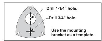
Install the work light and break-thru plug to the mounting plate. Pass the electrical connector through the provided break-thru plug and connect to the provided wiring harness. Install the harness into the 1-1/4" hole, then install the mounting plate to cover the two drilled holes.
