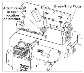
Electrical enclosure covers and relay/fuse assembly wires not shown.
