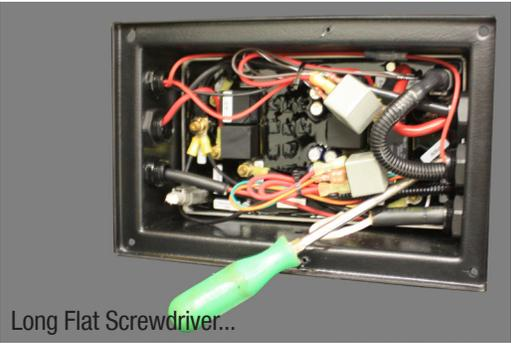
Step 7: Remove the Connector Cap located in the lower left-hand corner of Control Module Box.
