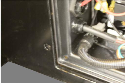
Step 10: Tighten the Harness Restraint of the Salt Traxx Harness. Re-Install Control Box Cover and Auger Extension Cover.
