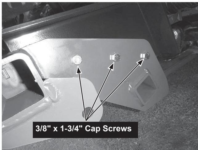
Secure the cap screws with  $3/8$ " washers and  $3/8$ " locknuts. Hand tighten the fasteners. Repeat on the passenger's side.
