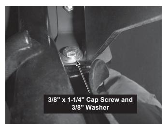
5. Repeat Step 4 on the passenger's side to install the passenger-side bracket.
