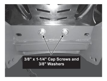
4. Fasten the driver-side bracket to the skid plate assembly using two 3/8" x 1-1/4" cap screws. A 3/8" washer must be used on both sides of the slotted hole. No washers are necessary on the bottom bracket/skid plate assembly hole. Secure with 3/8" locknuts. Hand tighten.
