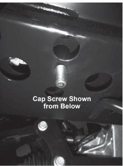
3. Install a hanger assembly over the 1/2" cap screw from Step 2. The cap screw should protrude through the middle hole of the hanger. Secure with a 1/2" locknut. Hand tighten.
