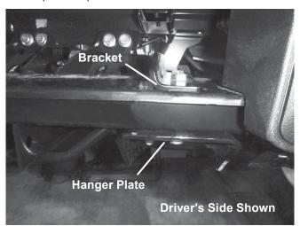
7. Install a 1/2" x 1-1/4" cap screw on handle into the frame on the passenger's side. Insert the fastener through the frontmost hole; bend the handle as necessary. Install a second cap screw on handle farther into the frame and through the second hole rearward from where the first cap screw on handle was inserted.
