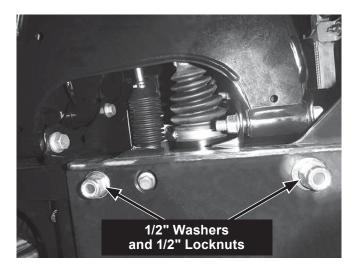
10. Fasten the skid plate assembly to the hanger brackets using two 1/2" x 1-1/4" cap screws on each side. Secure with 1/2" locknuts and hand tighten.
