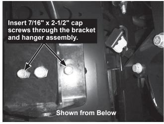
5. Tighten the 7/16" x 2-1/2" cap screw and the 1/2" x 1-1/4" cap screw installed in Step 2 according to the torque chart. The top of the 1/2" cap screw is accessible through the back of the winch plate.
