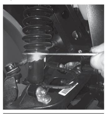
NOTE: After five to ten hours of snowplow usage, retorque all mount assembly fasteners.
