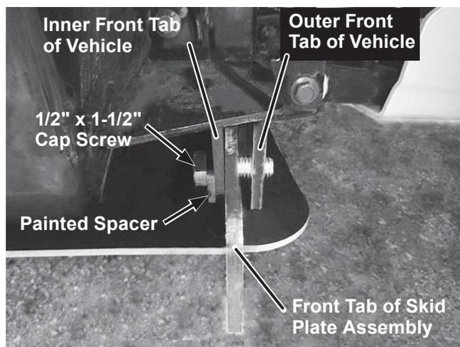
4. Secure the fasteners installed in Step 3 using 1/2" locknuts, placing the locknuts in the openings of the vehicle's outer front tabs. Hand tighten only.
