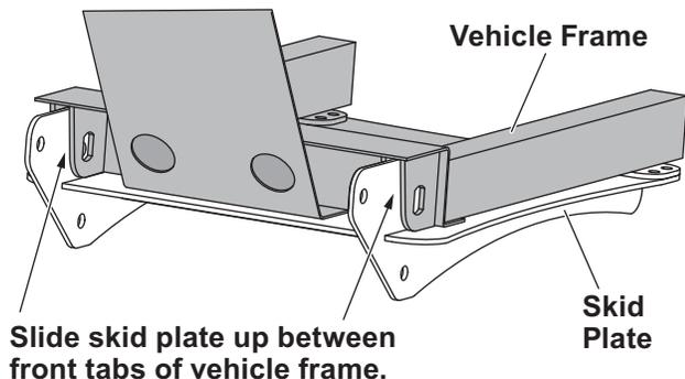
Install the 1/2" x 1-1/2" cap screws with spacers from Step 2 through the inner front tabs of the vehicle and front tab of the skid plate assembly.
