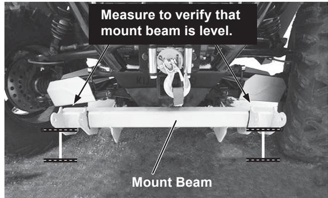
14. Measure the distance between the mount beam rear hole and the ground. If it exceeds 11-1/2", install the accessory Height Adapter Plate Kit (PN 77555) to ensure optimum plowing performance.
