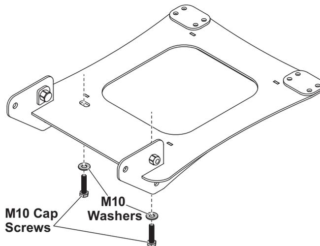
6. Center the mount from left to right. Clamp the rear of the skid plate assembly to the vehicle frame.
