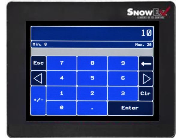
Enter the desire time you would like the discharge pump to run. (Min. 8 minutes – Max 20 minutes)
