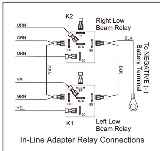
**NOTE:** If ring terminal wire does not reach battery, lengthen wire as required.
