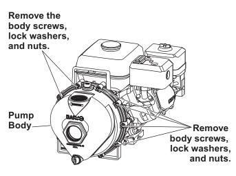
2. Remove the check valve from the volute. Remove the one upper and two lower volute screws, and remove the volute. Save all for later use.
