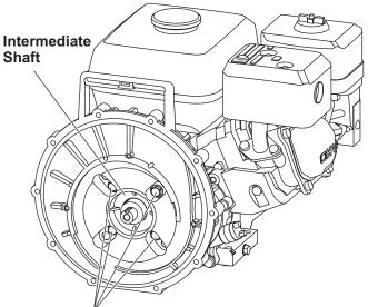
Rémove 4 bracket screws, rear bracket washers, and screw head O-rings. 7. Using a round object such as a wrench socket, tap gently with a hammer to remove the carbon seal half from the rear bracket. The seal is very fragile; take care not to crack the seal if it will be reused.
