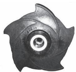
Install the impeller key shaft and impeller onto the engine drive shaft. Secure the impeller to the drive unit shaft with the impeller bolt gasket and the 5/16" x 1-1/8" hex flange cap screw. Tighten the cap screw until snug.
