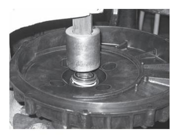
8. While the pump is completely disassembled, clean all of the reusable parts thoroughly, removing any traces of old gasket material and trapped or dried liquids that were run through the pump.
