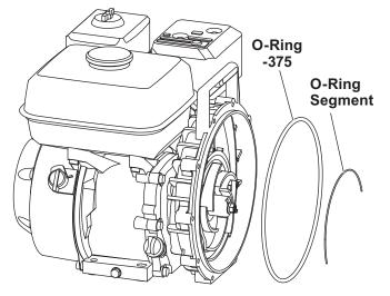
7. Reinstall the volute onto the rear bracket using the three volute screws. Reinstall the check valve onto the snout of the volute. The drive unit should be turned over a few times to check for clearance between the impeller and volute. A small amount of drag between the impeller and volute will cause no problem; however, if the drive unit will not turn over because of the lack of clearance, a shim may have to be used.
