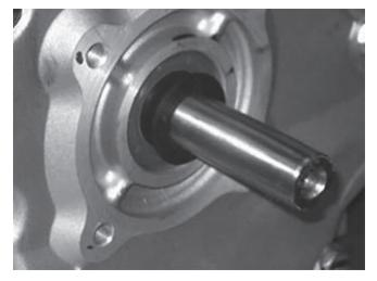
Place the seal O-ring behind the lip of the spring half of the seal assembly. Install the seal assembly half into the rear bracket using a tool such as a 1-1/2" pipe nipple or arbor press to give even pressure on the metal flange of the seal housing during installation. Gently press the seal into position until it bottoms.
