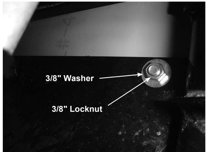
2. Install four 3/8" cap screws through the holes in the front of the skid plate assembly. Secure with a 3/8" washer and locknut, and hand tighten.
