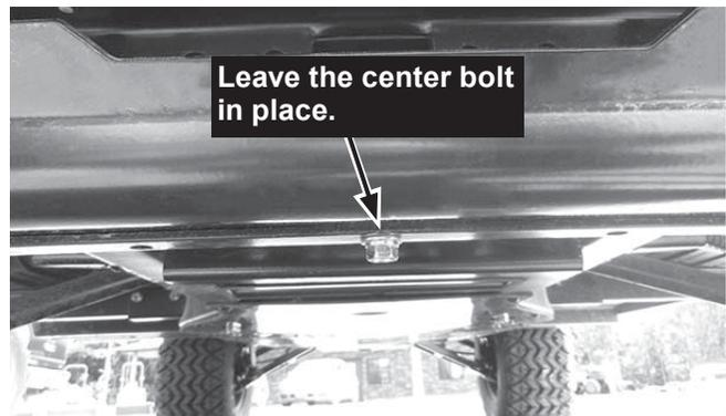
3. Insert two 3/8" x 5" cap screws into each rear bracket. Place the brackets over the frame, one on each side of the vehicle in the location shown.
