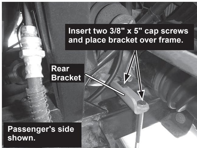
4. Place the skid plate assembly against the bottom of the vehicle, allowing the cap screws from the rear brackets to protrude through the corresponding holes in the skid plate. Align the center hole of the skid plate assembly with the center bolt left in place from Step 2.
