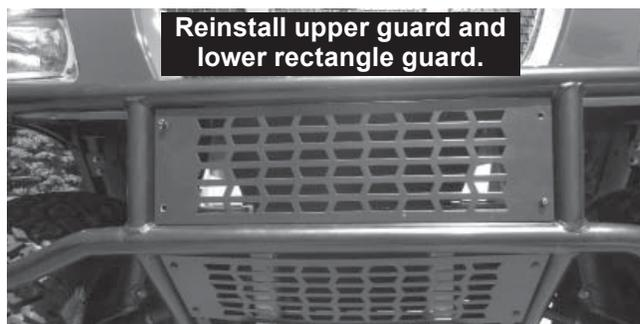
**NOTE:** After five to ten hours of snowplow usage, retorque all mount assembly fasteners.
