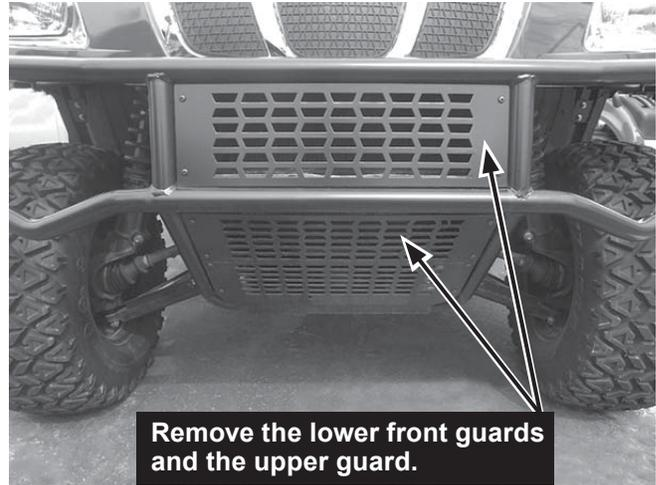
2. Remove the left and right lower brush guard assembly bolts found underneath the vehicle. Leave the center bolt in place.
