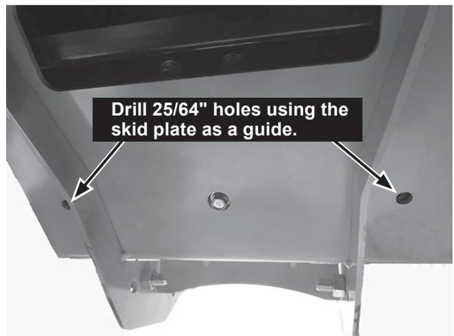
12. Insert 3/8" x 1-1/4" cap screws through the holes drilled in Step 11. Secure with locknuts; hand tighten.
