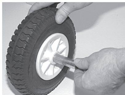
Push the sleeve through the wheel.
