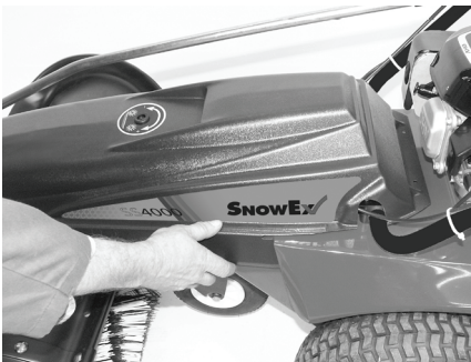
Set the brush at an angle. Slip the cover over the belt area and back so the Snap Nuts can be seen through the holes in the cover.
