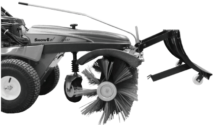
Hold plow at an angle, lower plow over receiver bar. The bar will fit between the tabs on the plow.
