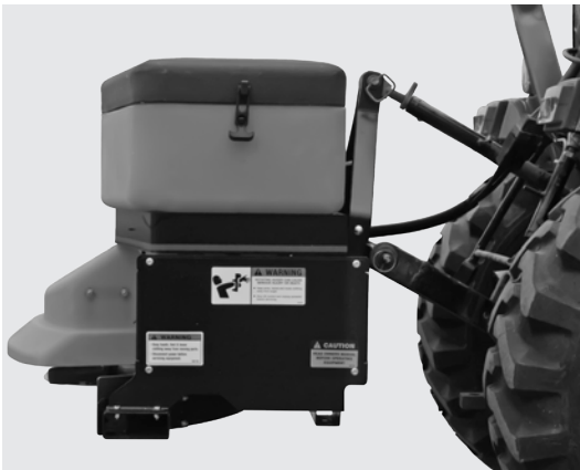
Adjust the top link so the Spreader is vertical.
