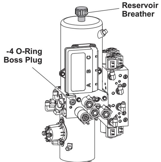
5. Install the pressure switch in place of the O-ring boss plug. Gripping the hex portion only, tighten the pressure switch to 10–13 ft-lb.
