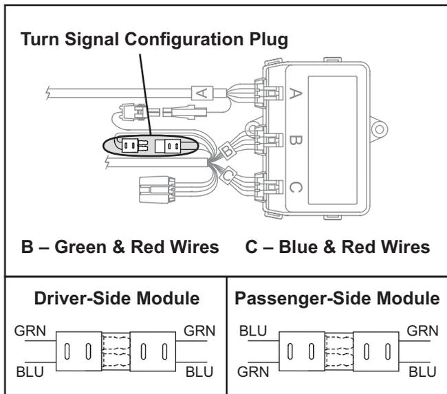
2. Complete the installation by securing the relay assemblies to an existing assembly with cable ties. Mount the relay connectors wire side down.
